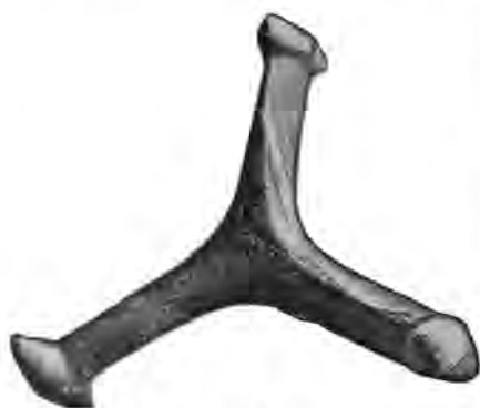
Stilt used in Modern China Manufactories From Trenton, N. J.
