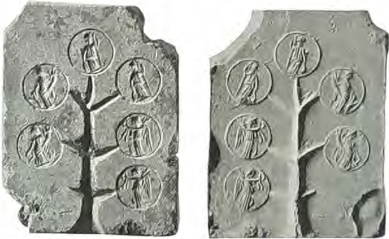
FIG. 214.—LIMESTONE HALF-MOULD, WITH CAST FROM SAME (No. 591). Ht. 4½ in.
